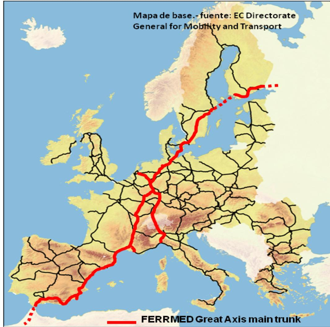
The main trunk of the FERRMED Great Axis Rail Network is so important for the EU that, in fact by 2020 in all its extension will have at least two parallel lines (not necessarily side by side) two tracks each.
